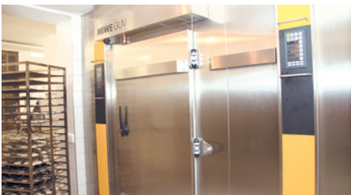
The GUV (left) is equipped with a TC control system, whereas the TLK works with FP control.
