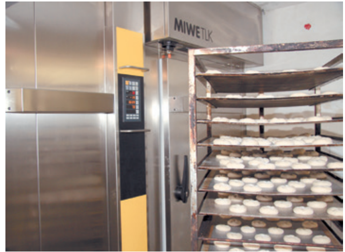
The TLK only requires a fixed programme control (FP) since hardly any programme changes are made here.
