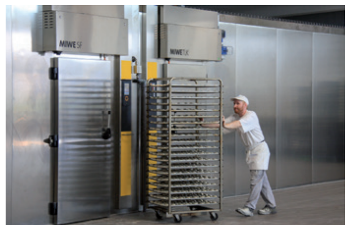
All dough pieces for deep freezing pass through the flash freezer, which significantly improves their quality.
