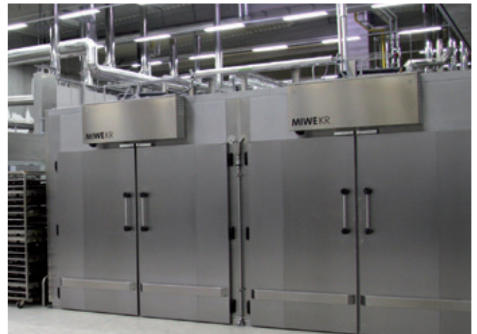
MIWE climatic chambers are available for proofing. They allow the temperature to be maintained precisely – even in hot summers – guaranteeing reproducible quality.
