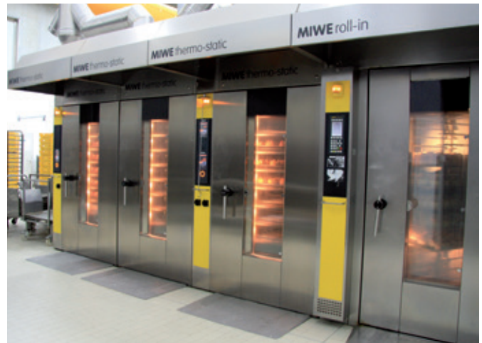
Thermal-oil wagon ovens and rack ovens are available for rolling loading.
