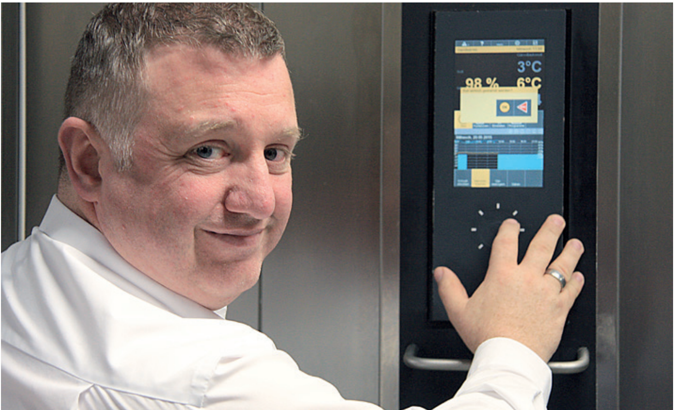
Marcus Staib wanted as few interfaces as possible at his new facility. The fact that the oven uses the same control system for the oven, refrigeration and heat recovery systems is an added advantage for Staib.
