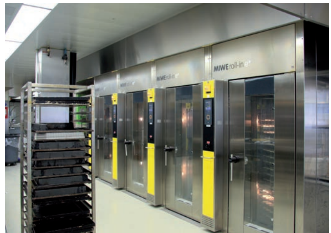
A total of 11 roll-in e+ units are fitted in blocks on the ground floor of the production facility.
