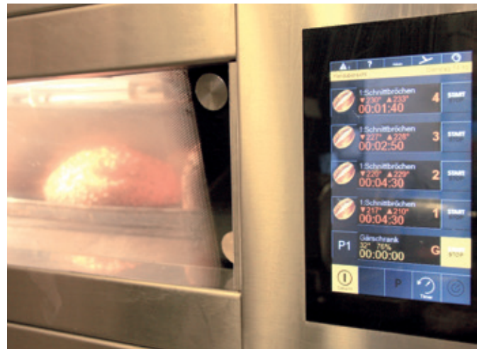
A single control system for all decks makes for clear and simple operation.
