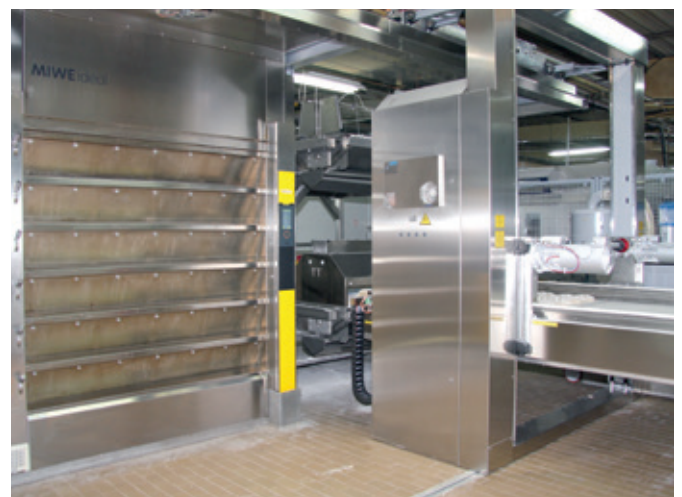
Loading unit MIWE athlet in front of the MIWE ideal.
