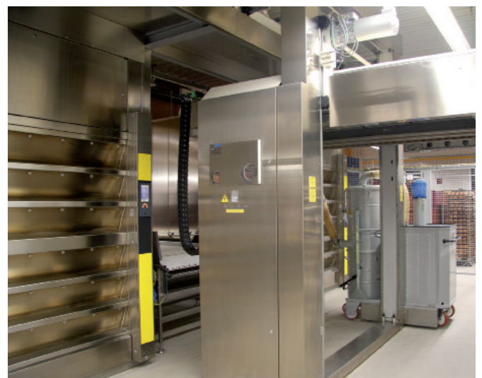
The two MIWE ideal ovens are loaded by a MIWE athlete. Between them, the conveyor to the dispatch area.
