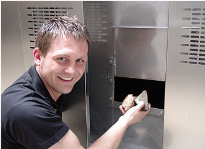
The eco:nova cleans the flue gases of sulphur dioxide. Christian Braun from MIWE shows us the limestone that is used in the neutralisation process.
