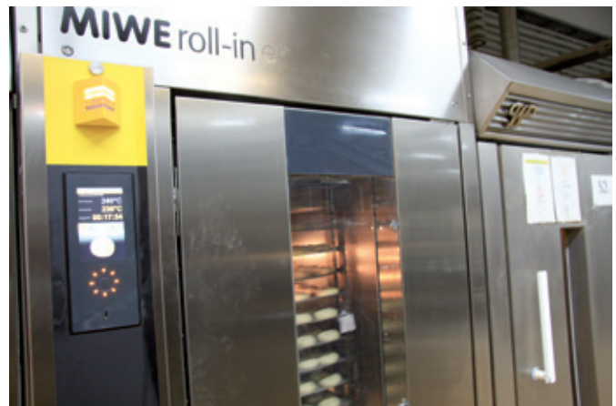
The MIWE roll-in oven’s control system is positioned separately, away from the hot baking chamber.
