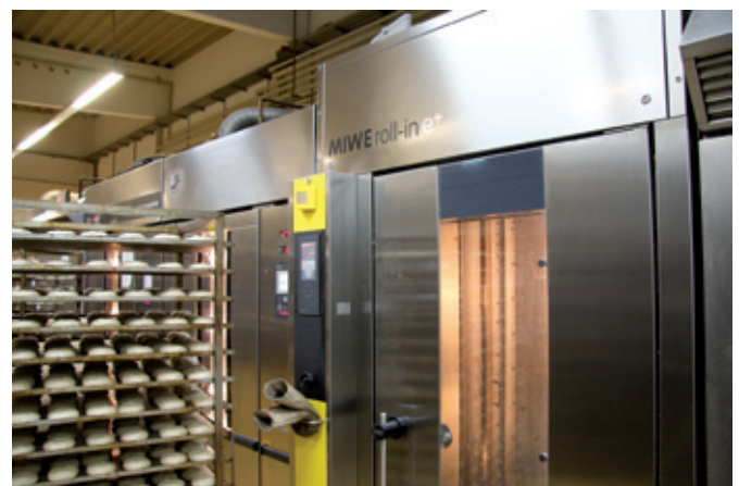
The heating phases for back-to-back baking are very short.
