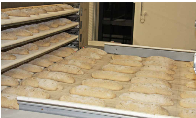
The MIWE athlete automatically pulls the baked goods from the loader belt onto its loading bar.
