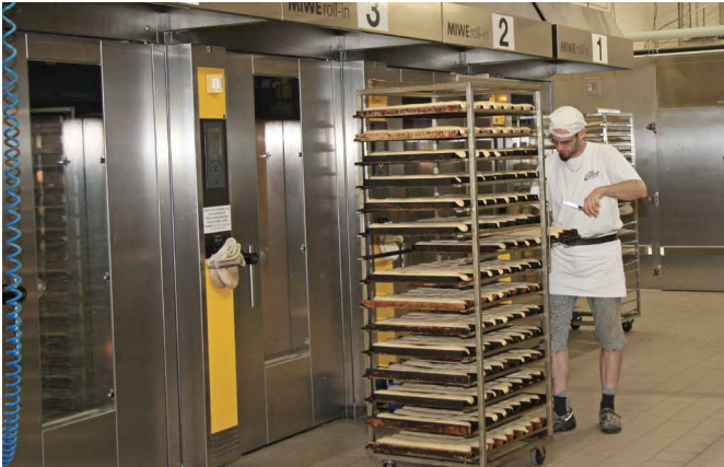
Working with the MIWE roll-in rack ovens.
