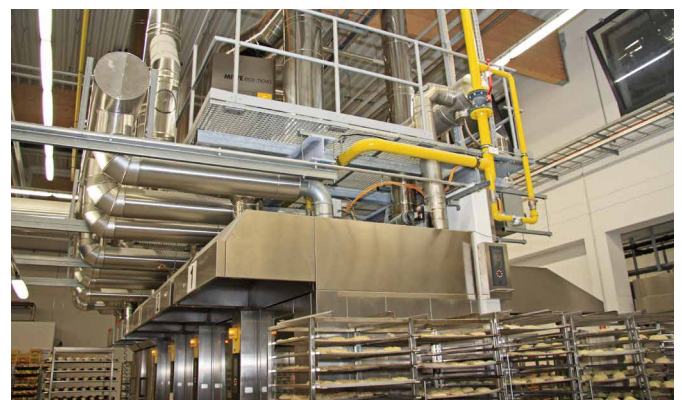
The MIWE eco:nova is built onto the rack ovens.
