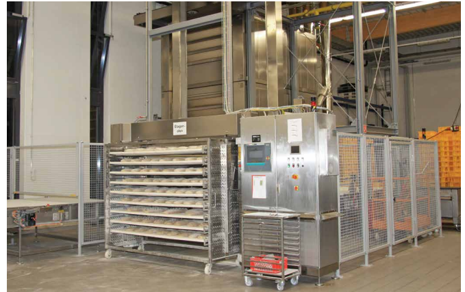
The MIWE butler working with a proofing trolley.
