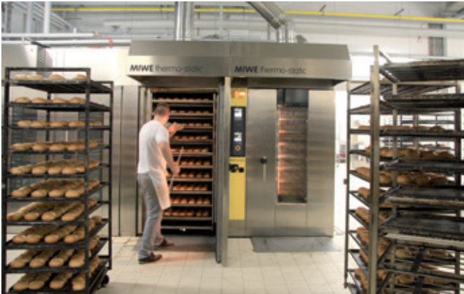
The two MIWE thermo-static are used for baking tin loaves and especially hard rolls.
