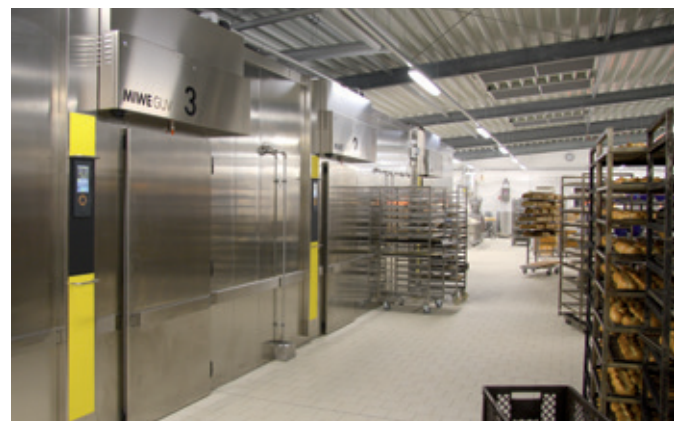
The cooling cells are situated across from the row of ovens. If heat is required, for example for defrosting or proofing, it is generated through a heat recovery process.
