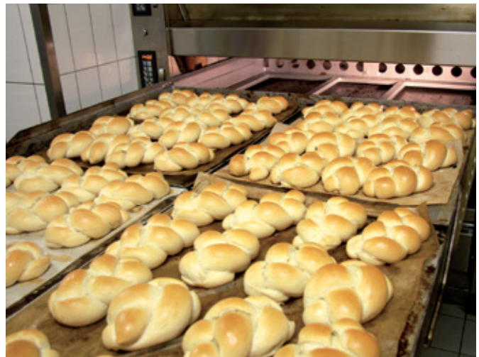
The draw-plate ovens make it easy to load and unload the ovens.
