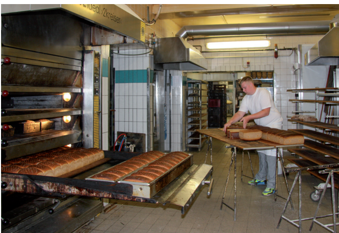
Large sets of moulds, like those for Paderborner bread, are baked on the draw-plate ovens in the MIWE ideal.
