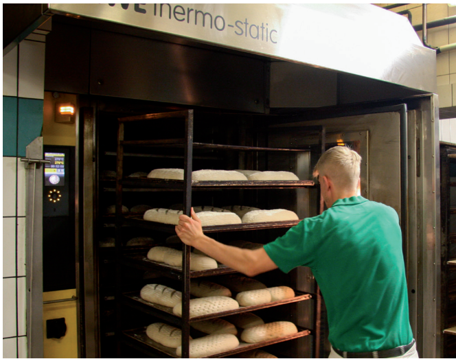
Where a deck oven used to stand, there is now a MIWE thermo-static with a directly integrated central heating boiler.
