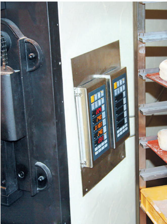
The control system for Wenz 1919 is installed on the side and thus not visible for the customers.
