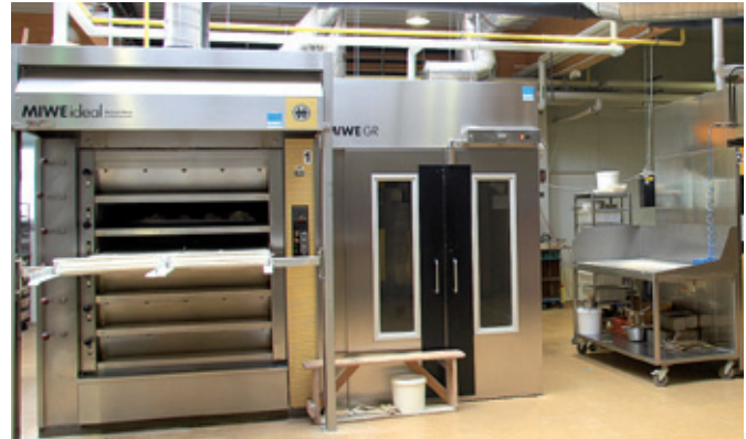
View of oven assembly comprising MIWE ideal deck oven, proofing chamber and rack oven.
