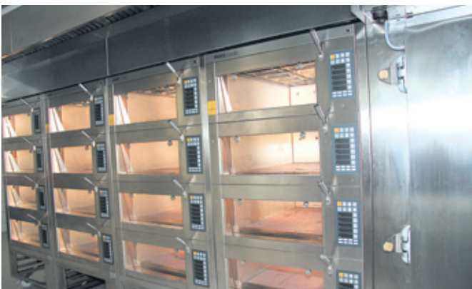
The control system for each oven is connected to a network and can be operated from the preparation room used by the teaching staff.
