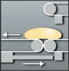
Synchronous transfer – ideal for soft dough, trays, tins and dough pieces on foil
