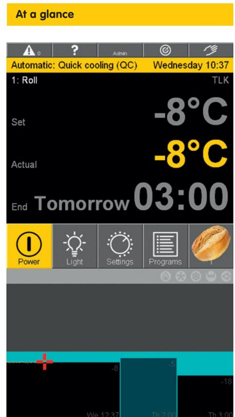
The main display of the MIWE TC: Efficient and with a clear layout, it displays all parameters in graphic or alphanumeric form. The black blocks stand for the individual phases with the respective setpoint setting; the yellow graph shows how the MIWE TLK converts the setpoint values into actual temperatures in real time, whereas the blue graph shows the humidity.
