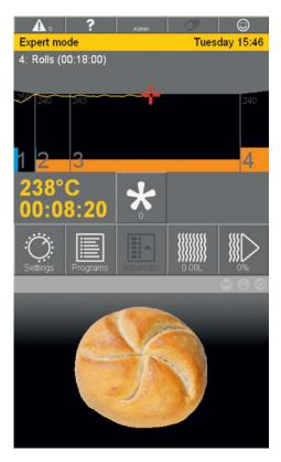
This mode provides all baking parameters graphically and/or alphanumerically in an efficient, clear manner. The black blocks stand for the individual baking sections with the respective setpoint setting; the yellow graph shows how the oven converts the setpoint values into actual temperatures in real time. Steam appears in blue at the precise time, and the water volume is displayed to the precise deciliter during steam input. Orange bars show use of the two-level turbosystem.
