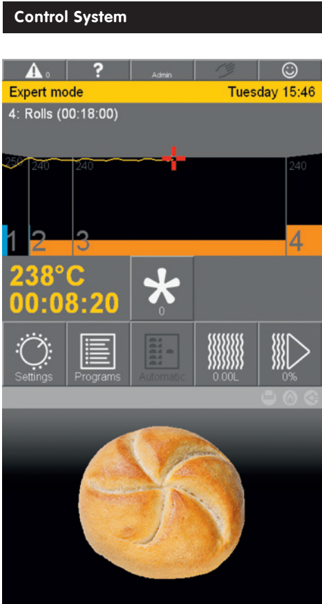
This mode provides all baking parameters graphically and /or alphanumerically in an efficient, clear manner. The black blocks stand for the individual baking sections with the respective setpoint setting; the yellow graph shows how the oven converts the setpoint values into actual temperatures in real time. Steam appears in blue at the precise time, and the water volume is displayed to the precise deciliter during steam input. Orange bars show use of the two-level turbosystem.
