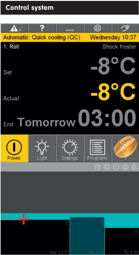
The main display: Efficient and with a clear layout, it displays all parameters in graphic or alphanumeric form. The black blocks stand for the individual phases with the respective setpoint setting; the yellow graph shows how the MIWE SF converts the setpoint values into actual temperatures in real time, whereas the blue graph shows the humidity. You will find other screen shots on the last page of this product information.
