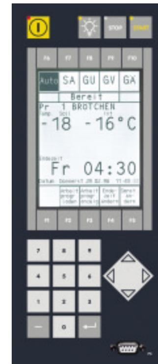
Combined system includes flash freezing, freezing, dough storage unit, proofing retardation, and proofing interruption and retardation
