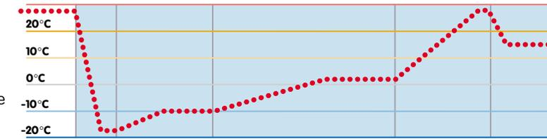
▲ Temperature range of MIWE GVA Fully-automatic Proofing Unit
