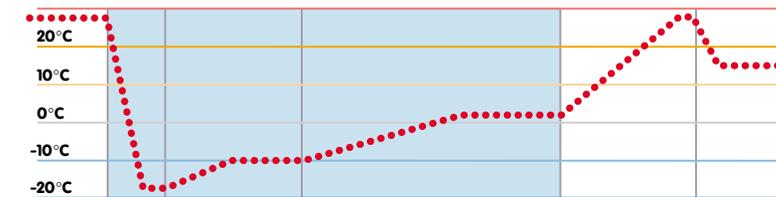
▲ Temperature range of a MIWE GUV Proofing Interruption and Retardation Unit
