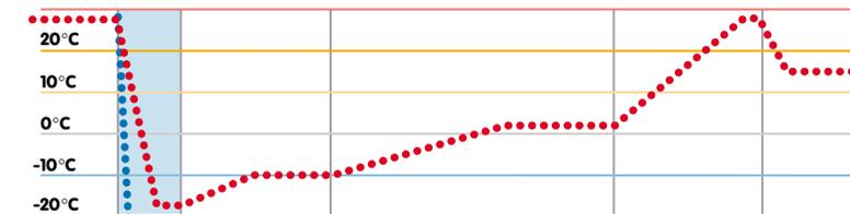
▲ Temperature range of a Flash Freezer (red = temperature curve GVA)
