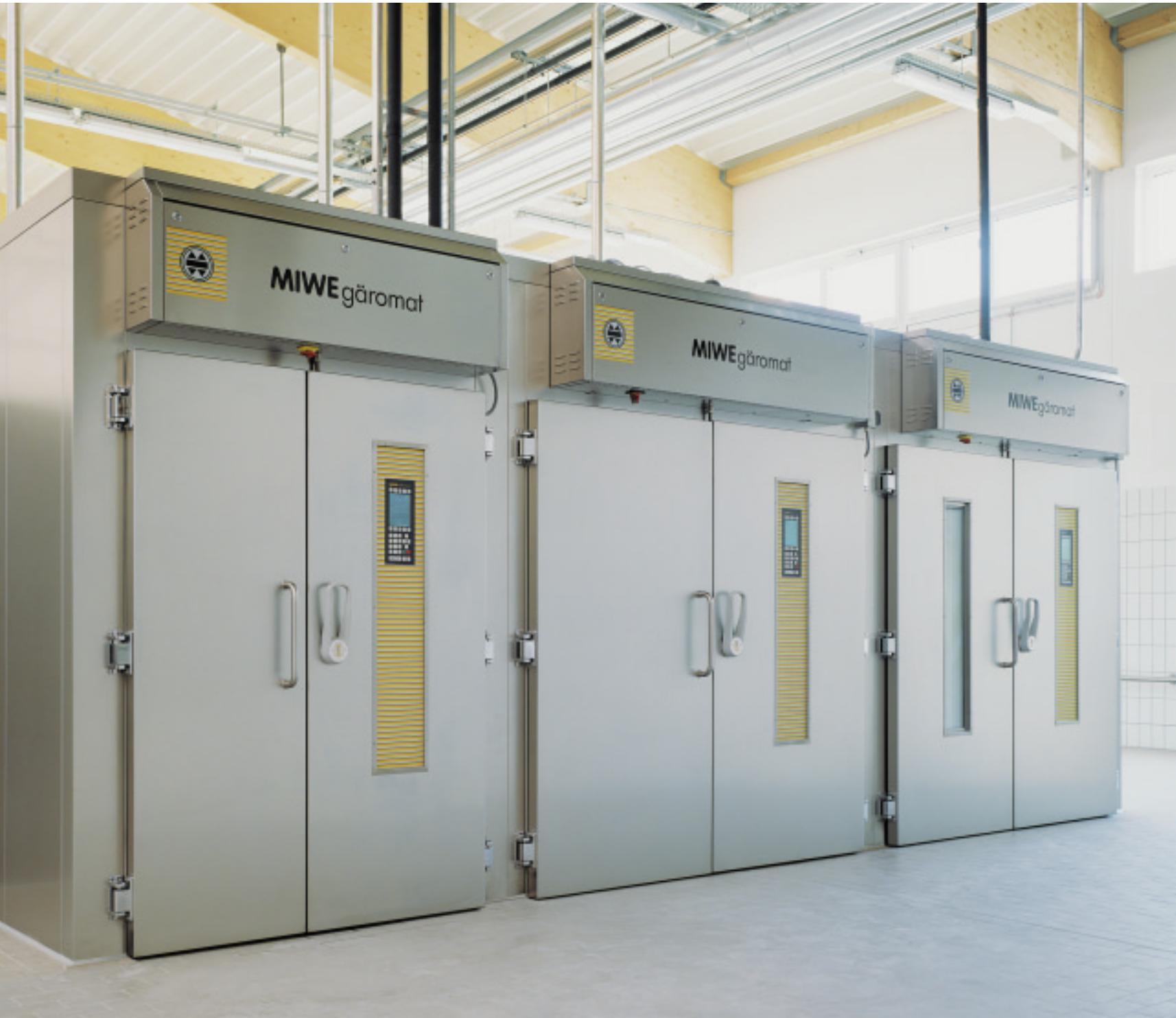
A sophisticated, user-friendly system: two rows of ventilators (right) ensure a precision-driven flow of air as of the fully-automatic proofing unit (GVA) and the proofing and retardation unit (GUV); easily-removable pressure walls (below) make regular cleaning a breeze.
