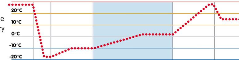
▲ Temperature range of a MIWE GV Proofing Retardation Unit
