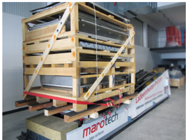
Braking simulators with heavy ovens at the European load safety competence centre
