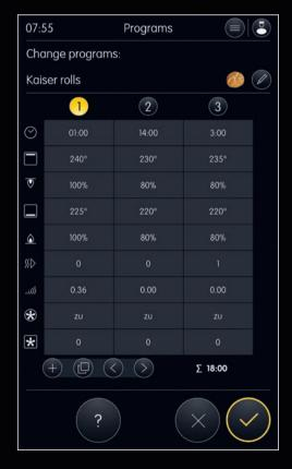
Creating baking programs? Nothing is easier! In the table view of all parameters, it is sufficient to click on the respective box in order to enter or change the respective value.
