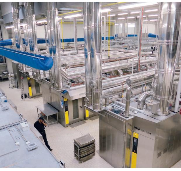
MIWE eco:nova, which recover as much of the technically inevitable waste heat in baking processes as possible with maximum efficiency and intelligently re-use the recovered energy in the bakehouse. Comprehensive monitoring (e.g. via
