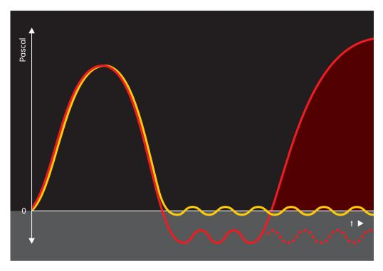
After the first supply of steam, the pressure drops into the "uncontrolled area" (grey zone), depending on the environment. It stays there until the end of baking (dotted in red) or shoots up again (red line) after the slide valves are completely opened.
