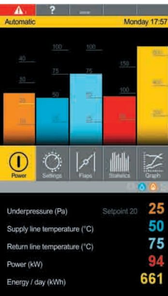
The touch screen of MIWE eco:nova clearly shows you how much energy you can recover by the hour, day, and year.
