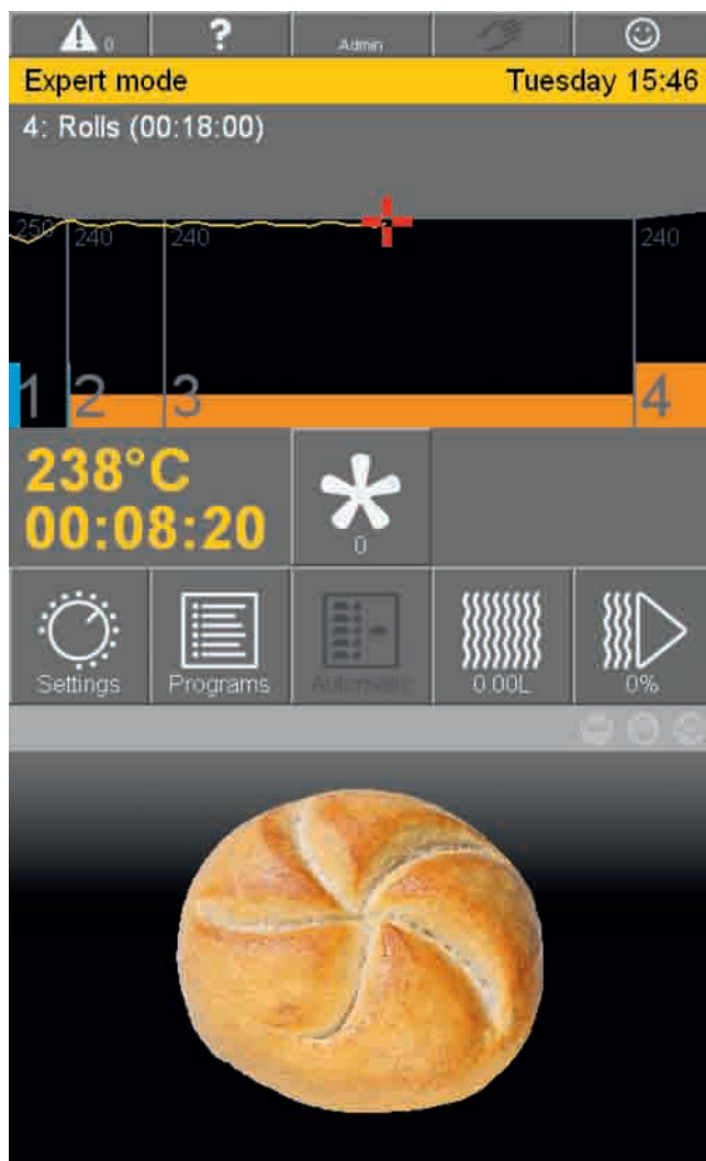
Always a clear view: the orange bar defines the use of the two-stage turbo system – the blue bar indicates the steam input.
