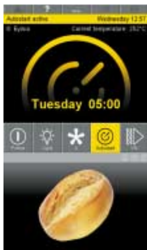
Images from top to bottom: Start-up screen, programming of night start-up times, „screen saver display“ with programmed night start-up.
