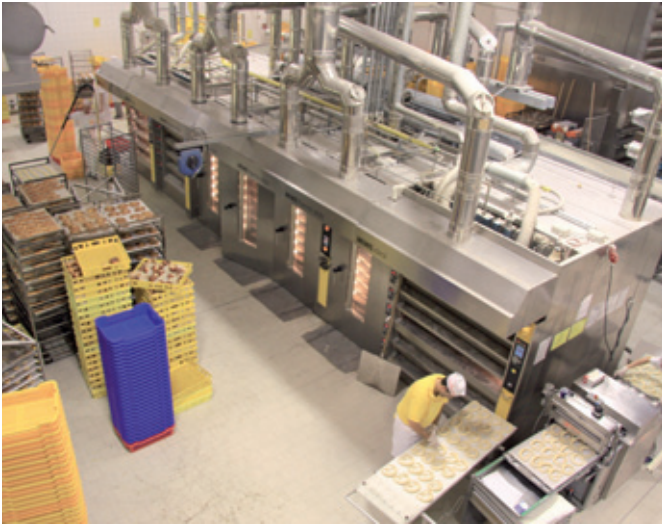
View of the ovens: wagon oven (centre) and deck baking ovens (left and right).
