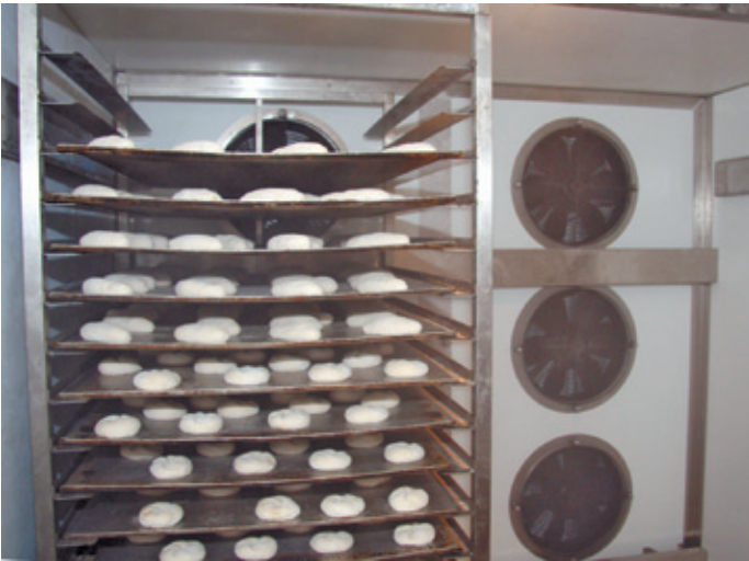
There is a quick cooling unit for two rack trolleys integrated into the TLK.
