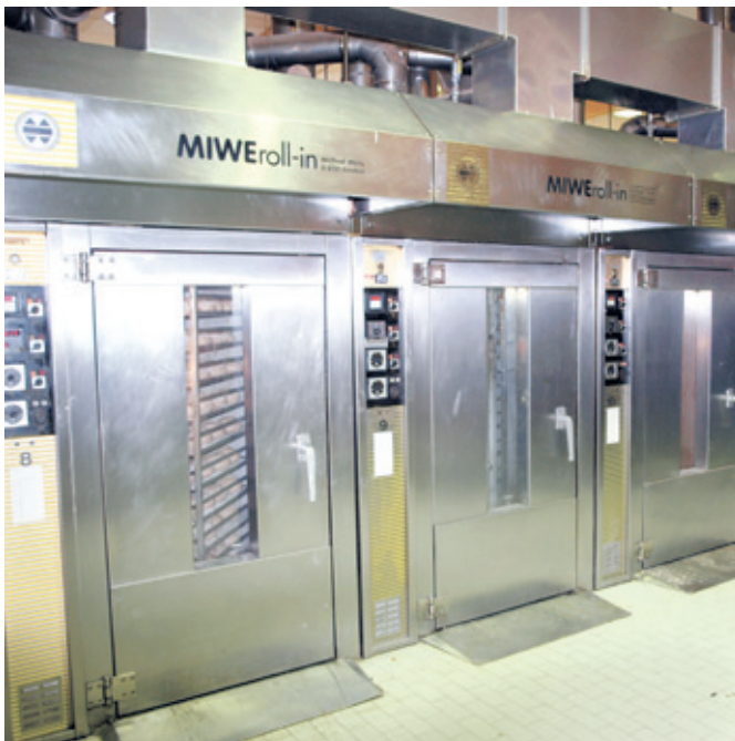
At Werner, the rack ovens are installed as an island. Five on the one side, five on the other. One bakery, and one pastry shop.
