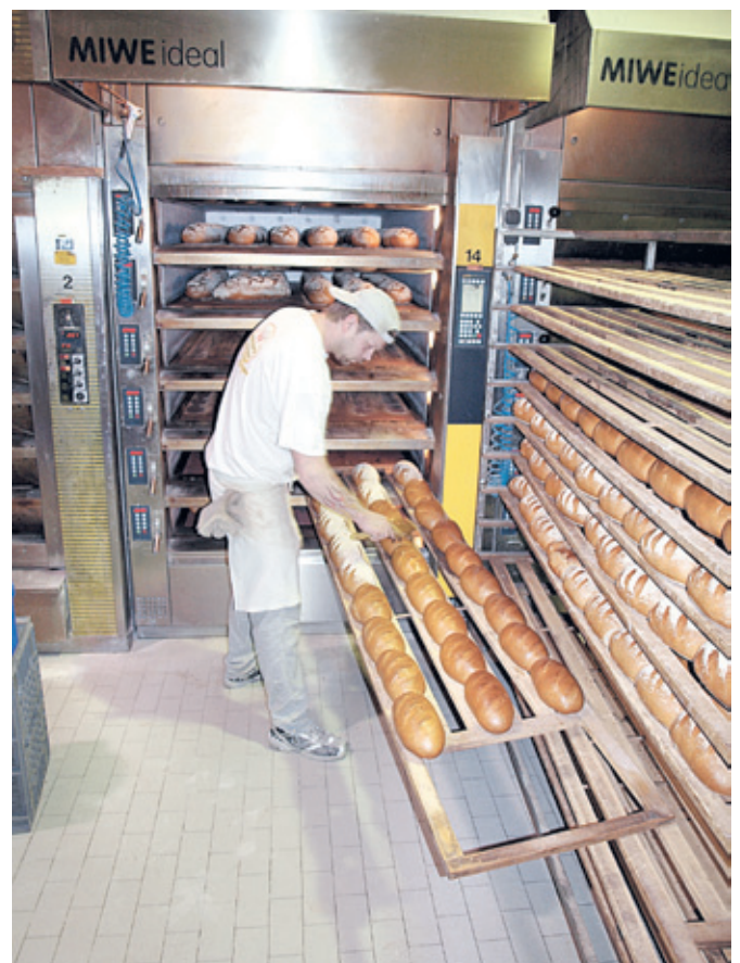
At Werner, the unloading is carried out with unloading boards; an automatic loading is not possible due to the different oven mass.
