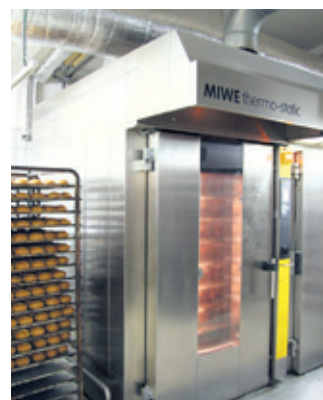
Baking like on a deck and loading like with a rack trolley: the thermal-oil baking oven combines the advantages of two worlds.
