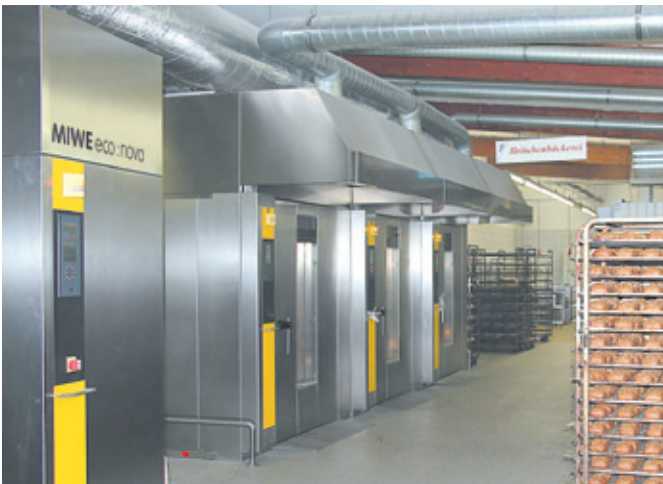
Constant operation concept: three double rack ovens and the new heat recovery unit MIWE eco : nova.
