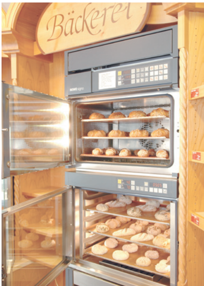
The MIWE in-store baking ovens are installed in the rear wall behind the counter. The proofing chamber is located beneath the two baking ovens.
