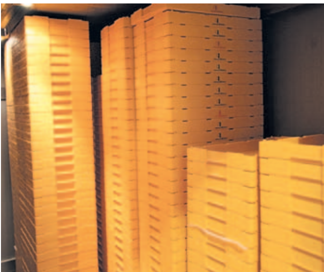
In contrast to the storage on trays or on normal boards, more dough pieces can be stored in the same room thanks to the special boards.
